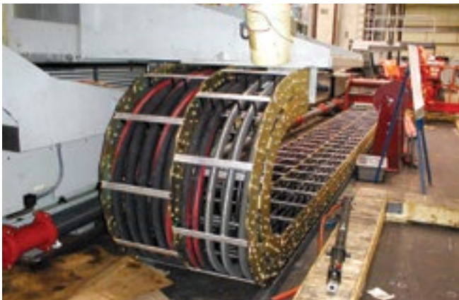
Nested Gortrac steel XL carrier system used on a large machining center for the aerospace industry.
