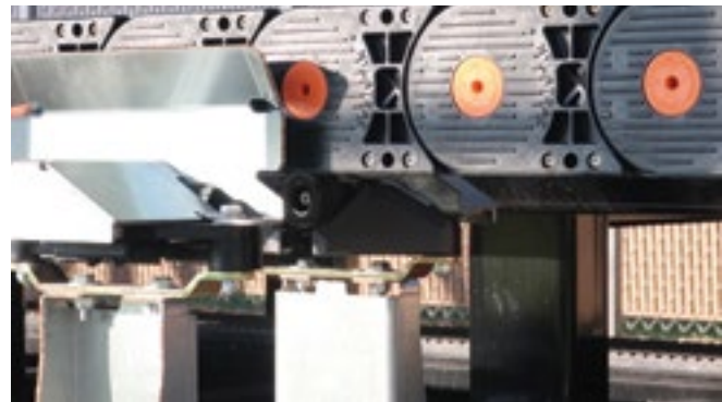
The ARS system eliminates the need for guide troughs and associated wear in travels up to 300 feet while reducing tow force and installation time by an average of 50%.
