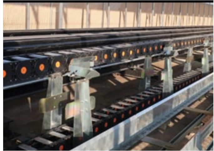
The ARS system eliminates the need for guide troughs and associated wear in travels up to 300 feet while reducing tow force and installation time by an average of 50%.
