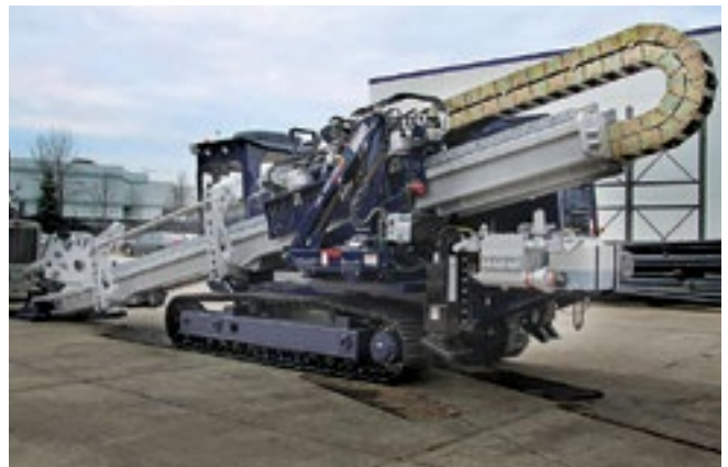
Nested Gortrac SRC Series carriers protect and guide hoses on this horizontal directional drilling machine by Universal HDD™.
