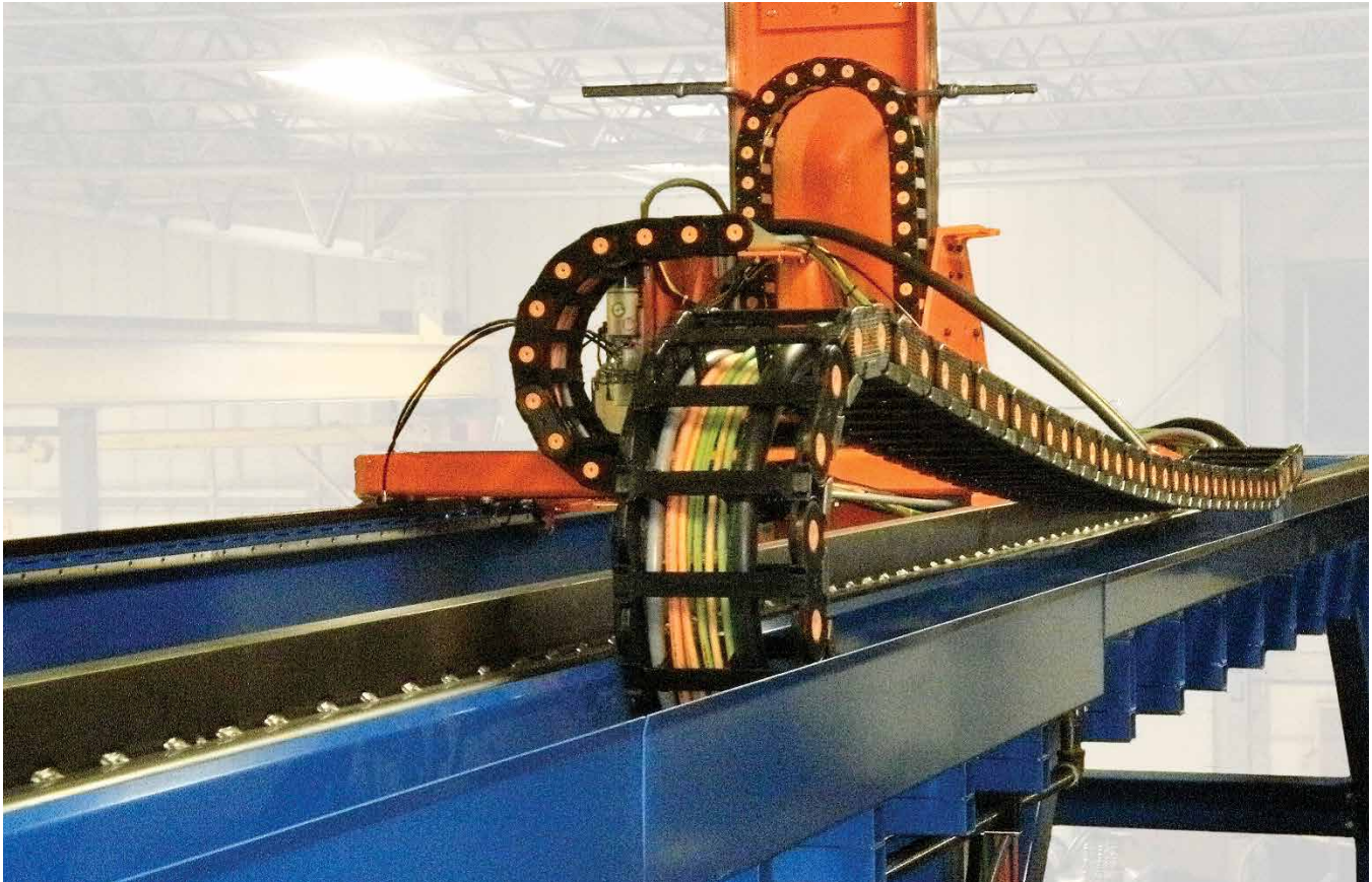
Nylatrac ® Modular TS and TSC carriers installed on custom pick-and-place equipment provide cable/hose management for long travel and three axis of operation.
