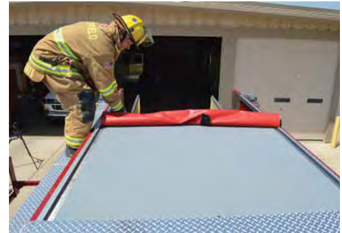
AFTER WITH GORTITE HOSE BED COVER INSTALLED
