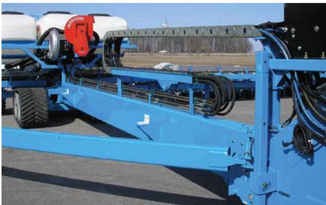
A steel Gortrac LRC Series carrier was customized for increased box strength to handle the vibration experienced by the carrier during operation. This planter with 88-foot wide extension allows greater coverage with fewer passes.
