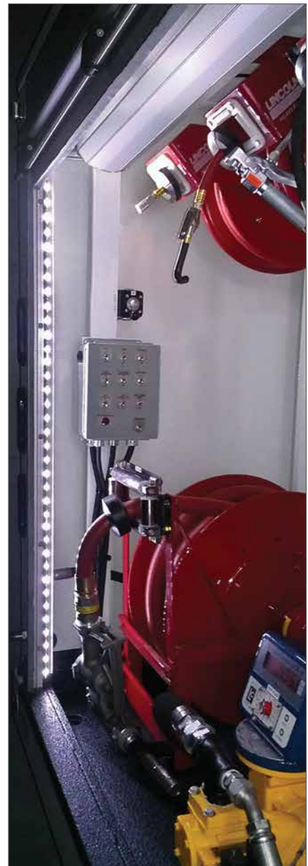
Gortite LED lights installed in aluminum rail channels illuminate the compartment in the dark.
