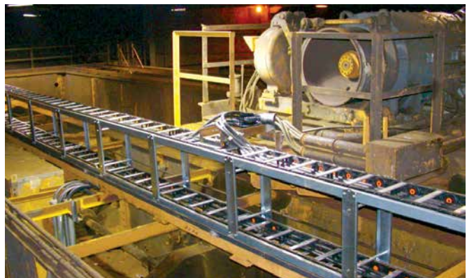
Shown: An opposed rolling carriage with a Nylatrac® Modular carrier (TS Series) designed for high-velocity/long travel in a steel mill.
