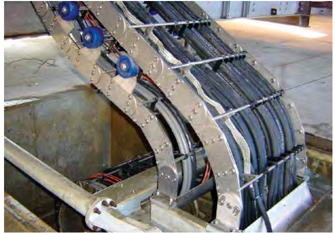
Custom stainless steel Gortrac ® LRC carrier system with rolling carriage for a rocket launch system in California. Driven end modified for customer's application requirements.
