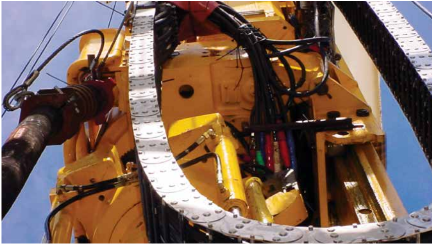
Custom 91-foot long Gortrac ® stainless steel LRC carrier maintains cables and hoses on an oil rig platform. Dynatect supplies many custom engineered carrier systems to the oil and gas industry.
