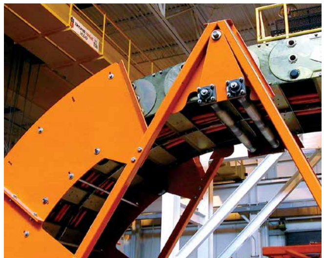
Blow-molding application with Gortrac steel XL carrier with patented "Walker" support system to reduce shock load by preventing link lock-out.
