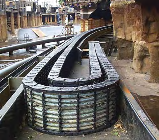
Nested Nylatrac ® Modular TL carriers operate fully submerged at an entertainment attraction. These carriers are designed for rotational and long travel in a side-mounted configuration.
