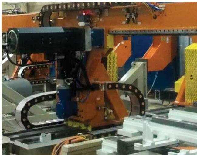
Nylatrac Modular TS carriers protect cables/hoses in multiple directions on high-speed servo-driven press transfer automation equipment. Bolted aluminum armor plates shield the utility package from debris in a metal stamping environment.
