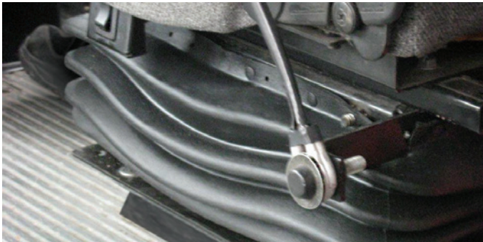
用于乘客座位调整的护罩 Bellows for driver's seat adjustment
