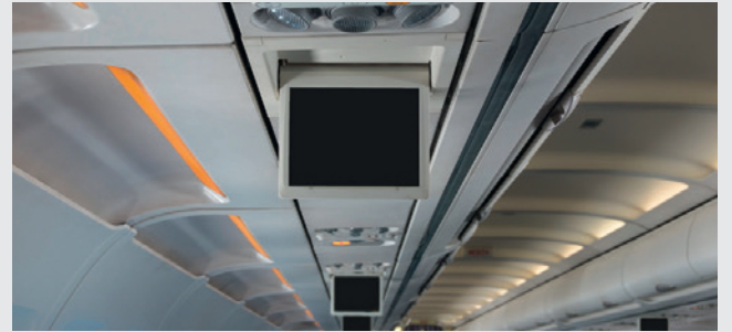
滑动式离合器用来在显示屏故障时保护驱动系统不受损坏，乘客不受伤害。 A slip clutch prevents drive system damage or passenger injury in the event the screen is obstructed
